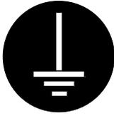
Connect the scanner and Ground with each other surely with the grounding wire. Otherwise, it is dangerous for you if you receive an electric shock or at the time of lightning. If the outlet does not have a Grounding Terminal or if it is impossible to connect, call the vendor or service professional for the installation.
